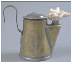
Tally lamps, such as this one, looked like miniature teapots. They used vegetable or animal fat and burned with an open flame. The hook attached to the miner's cap.
